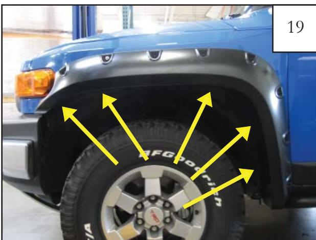
19 Position Flare on fender. Install five supplied Screws (SW1-0036). Do not tighten. *NOTE: It is helpful to install one of the top bolts first.*
